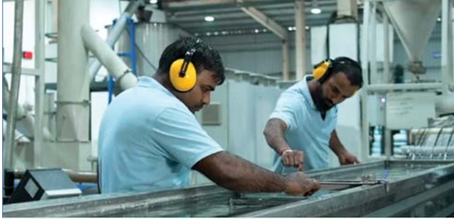
Employees overseeing the extrusion cooling process
